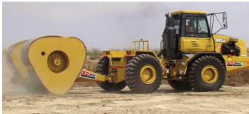
Figure 2-16. Rolling dynamic compaction (RDC)
